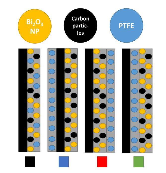
Experimental conditions: Catholyte: 0.5 M KHCO<sub>3</sub> CO<sub>2</sub> saturated Anolyte: 0.5 M H<sub>2</sub>SO<sub>4</sub> Electrolyte and CO<sub>2</sub> flow: 75 ml/min and 10 ml/min Mode: chronopotentiometry Geometric current density: -200 mA cm<sup>-2</sup> Time: 6 hours
