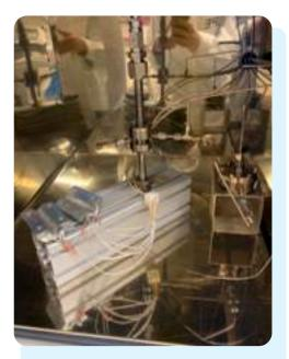
Figure 5 : Reactor for catalyst activity tests
