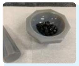
Figure 7 : Catalyst for the methanol synthesis
