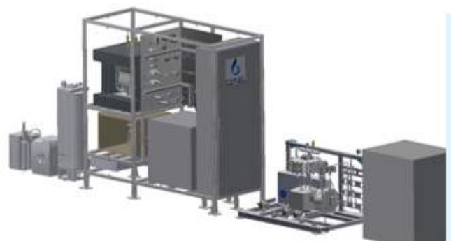
Figure 4 : 3D view of C2FUEL SOEC pilot
