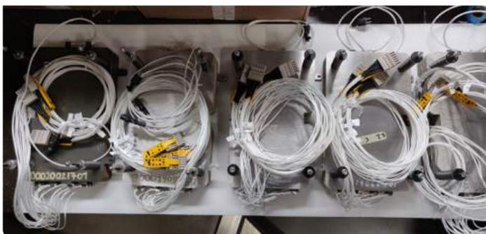
Figure 2 : SOEC stacks manufactured
