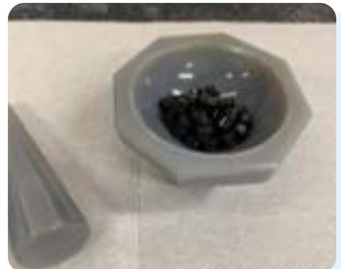
Figure 7 : Catalyst for the methanol synthesis
